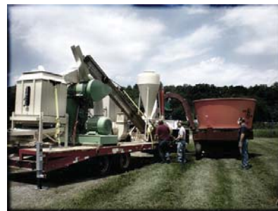
Mobile pelleting machine turns hay into pellets for energy.
