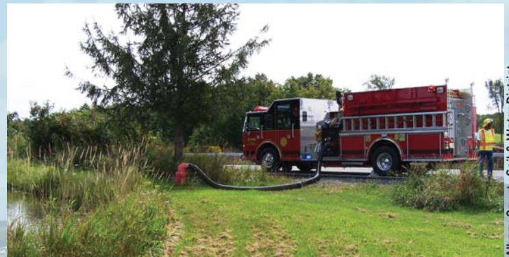
Soil and Water Districts work with local fire departments and highway crews to install cost-effective dry hydrants that are vital to saving lives and property in rural areas.
